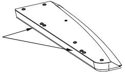
Place your bracket over the holes as pictured below and re-install the screws using the enclosed #8 washers (P30073-4) between the head of the screw and the bracket. Do this for both halves of the light, ensuring the brackets are mounted with the forks towards the outer edge of the light.
