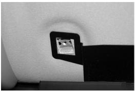
6. Align the square hole on the other end of the visor bracket with the visor clip hole.
