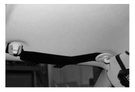
8. Tighten the screws on the visor arm to hold the visor bracket and light in place.
